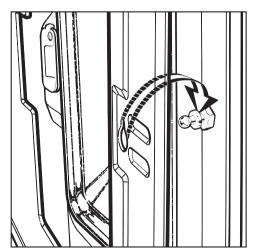
■ Ease the back lug into the opening in the rear wall panel.
